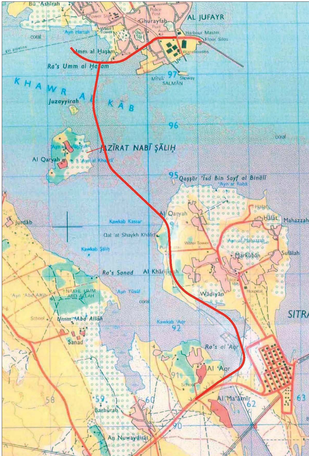
Topo map showing alignment of the causeway
